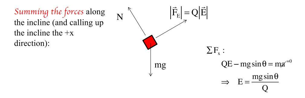
With the ELECTRIC FORCE up the incline, and remembering that negative charges feel FORCES *OPPOSITE* the direction of electric fields, the field must be DOWN the incline. If the +x direction is up the incline, we can write:
